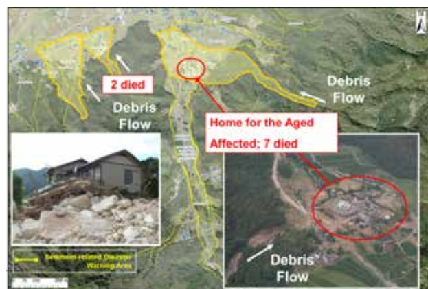
Fig. 2.3.2 Debris flows of the Yamaguchi disaster
