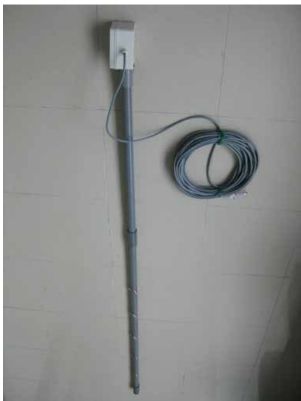
Water level gauge
