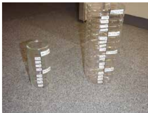
Fig 2.5.6 Simple precipitation gauges made of a glass and a plastic bottle
